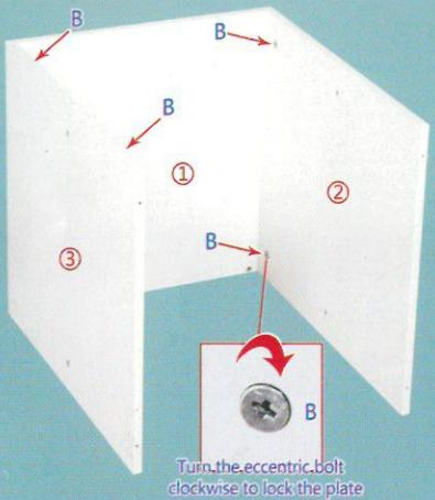
Turn the eccentric bolt clockwise to lock the plate
